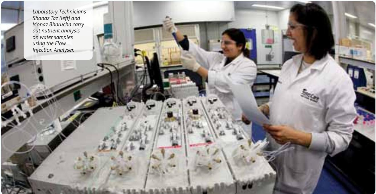
Laboratory Technicians Shanaz Taz (left) and Monaz Bharucha carry out nutrient analysis on water samples using the Flow Injection Analyser.
