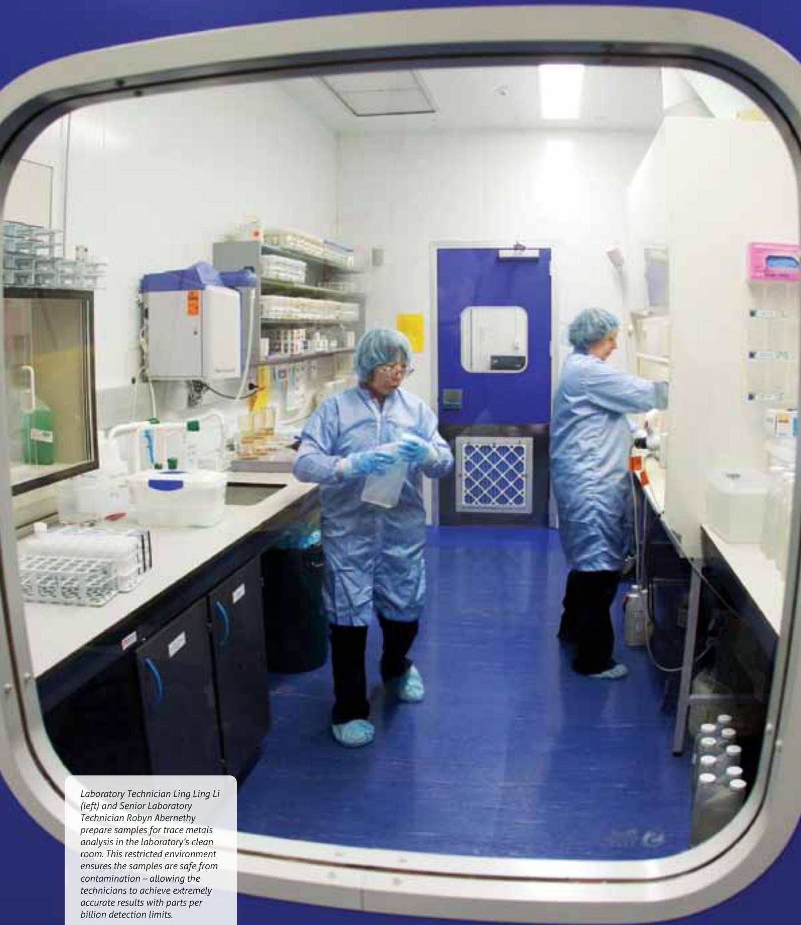
*Laboratory Technician Ling Ling Li (left) and Senior Laboratory Technician Robyn Abernethy prepare samples for trace metals analysis in the laboratory's clean room. This restricted environment ensures the samples are safe from contamination – allowing the technicians to achieve extremely accurate results with parts per billion detection limits.*
