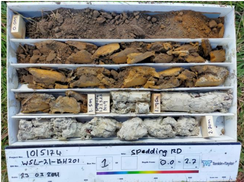
Figure 9. Borehole assessment carried out at the southern section of the BPC site. Results displayed to a depth of 2.7 m.
