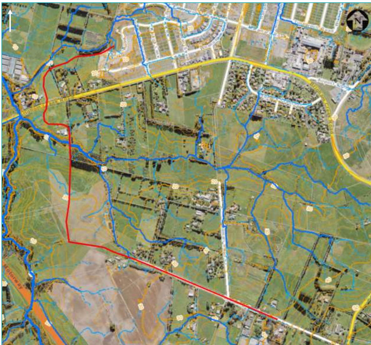
Figure 6. Contour information with overland flow paths – approximate site alignment shown as red line (Auckland Council Geomaps)
