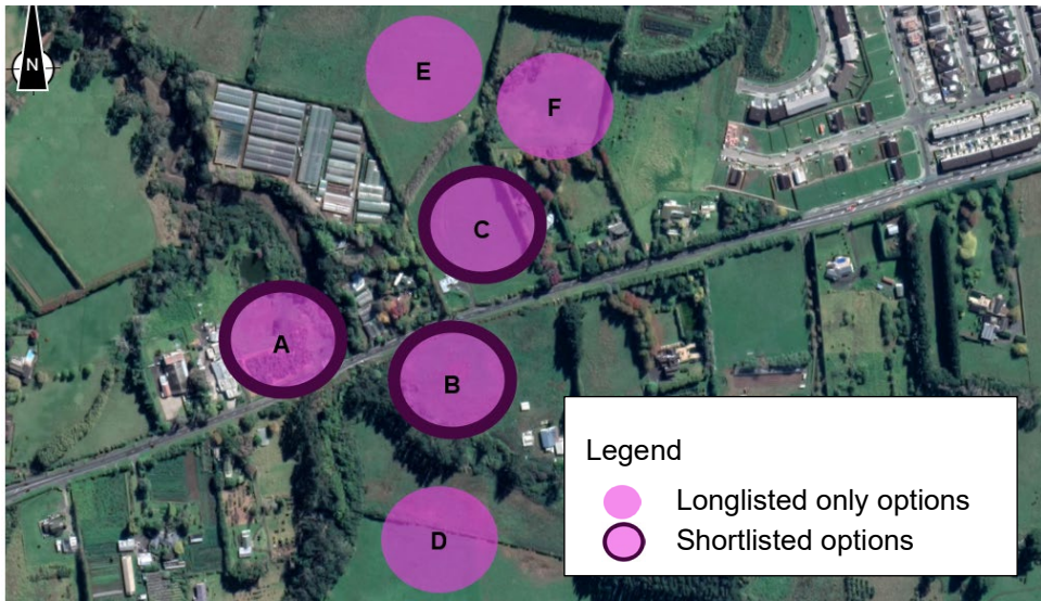
Figure 29. Pump station options considered
