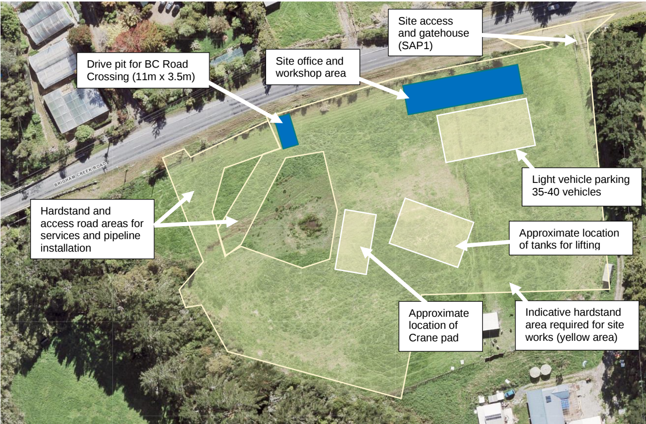
Figure 4-3. Contractor Area Hub Approximate Layout
