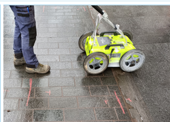
Figure 2 Underground services mark-out using Ground Penetrating Radar (GPR)
