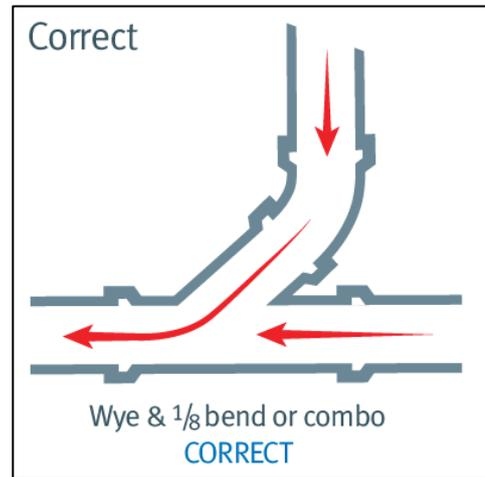
**5.3.10.1A Connections in combined stormwater and wastewater network areas**
