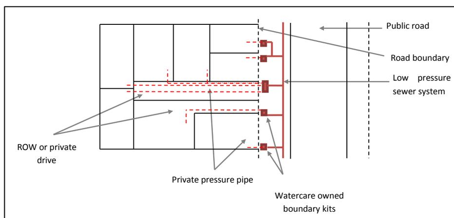
**Figure 5.1 Example of a low pressure wastewater system**
