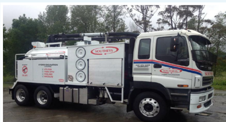
Figure 1 Vacuum truck or hand digging to identify and avoid underground services
