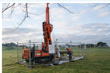
Figure 2 Drilling rig used to collect core samples. The rig may be supported by a four-wheel drive ute and a truck with a water bowser covering an area of approximately 15m 2
