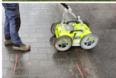
Figure 4 Underground services mark-out using Ground Penetrating Radar (GPR)
