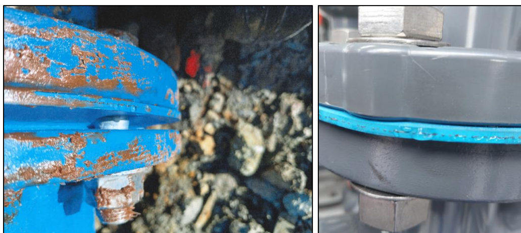
Figure 3: Field examples of reinforced EPDM gasket weeping water through reinforcement
