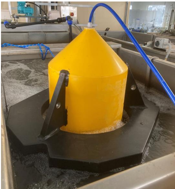
Watercare Innovation Centre – Prototype gas collection hood
