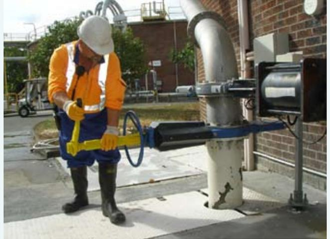
Plant Operator Nigel Prentice opens an isolation valve at the Mangere Wastewater Treatment Plant using a valve-exercising ratchet designed by him and Shift Engineers John Sutherland and Allan Julian. Their tool makes the opening and closing of these valves easy, whereas it used to take time and muscle power. The innovation was recognised with a Continuous Improvement Award.
