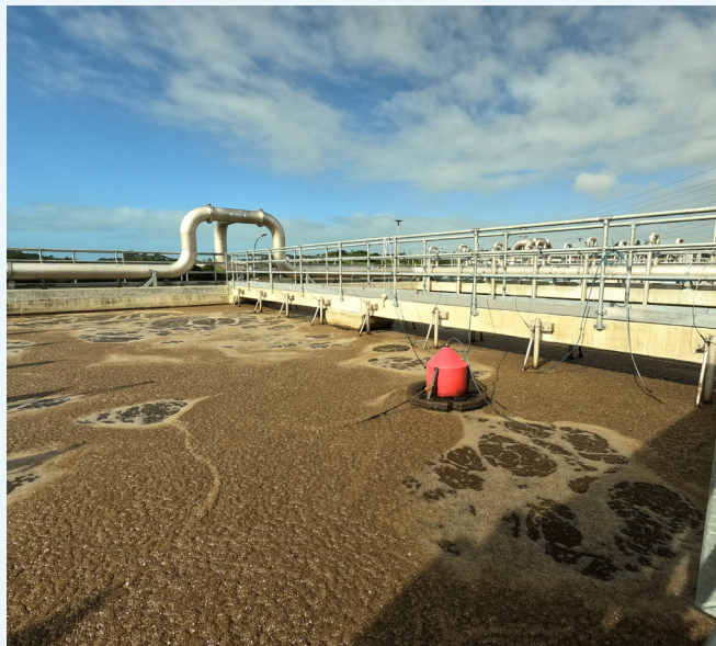
Greenhouse gas monitoring and analysis equipment – floating hood and Picarro unit. Rosedale Wastewater Treatment Plant.
